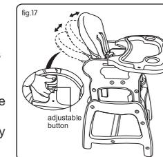
9. The backrest can be adjusted to 3 positions. To adjust backrest, pull up gently on the adjuster button on the back of backrest and move into the desired position.
