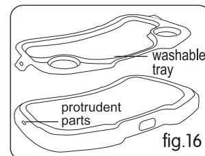
8. Slide tray into notches located on the outside of the armrests. A click can be heard when the tray is locked into place. To remove tray or move to another position press the adjuster levers on the underside of tray. The tray can be adjusted to 3 positions.
