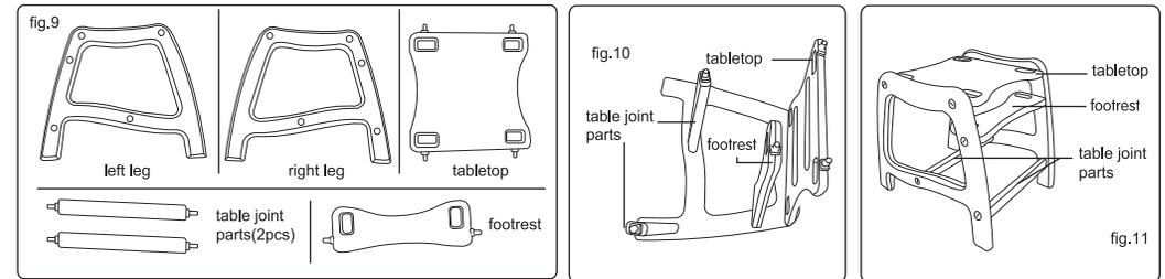
6. Insert the table top, table joint parts and footrest into the corresponding holes in the left and right table legs (fig. 10 & 11). Insert screws and tighten until locked.
