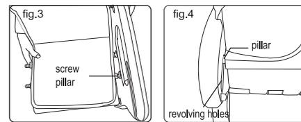
2. Put the two screw pillars, on the booster, into the corresponding holes in the left chair armrest. (fig. 3)
