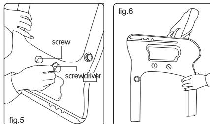
4. Insert screws through armrest into booster, using the screwdriver tighten until locked (fig.5 & 6)
