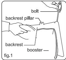
1. Join Backrest and booster together to create reclining hinge and place hinge bolt into axle holes. (fig.1)
