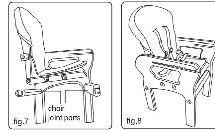
5. Insert the two chair joint parts into the corresponding holes. Please note: the shape of the protruding ends on the chair joints, matches with the holes in the armrests (fig. 7). Then attach right armrest as per steps 3 & 4.
